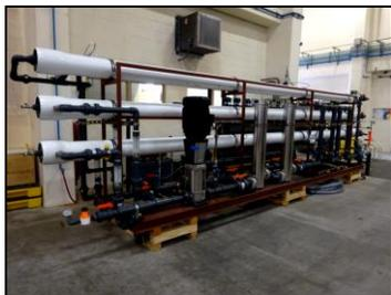
To facilitate pilot testing the City and MBC designed, permitted, and constructed a pilot unit that utilized full-size (8-inch diameter, 7-element) pressure vessels in a 2:1 array with independent cartridge filters and pre-treatment chemical feed systems. The pilot unit was permitted to withdraw feedwater from the NF process raw water header and discharge permeate and concentrate to the plant's respective headers.
